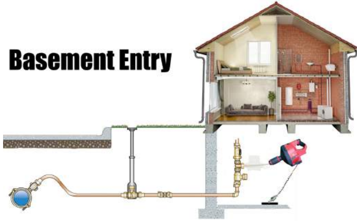
Figure 26. A Typical Basement Entry for SWORDFISH Survey.
