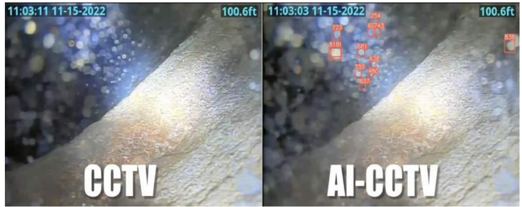
Figure 39. Electro Scan AI Uses High Resolution Cameras to Track and Confirm Leaks Found in Pipes.
