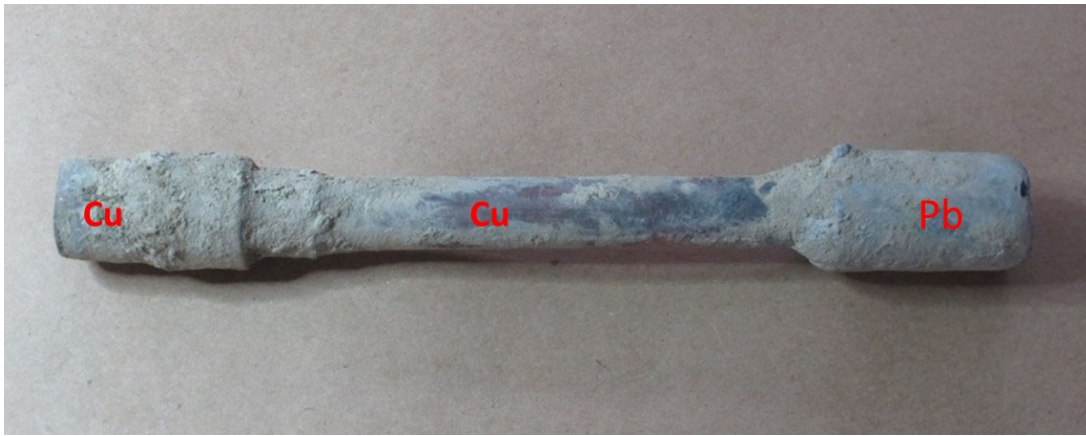
Figure A-7. Sample 16-0209-CP-3, Sample with Two Types of Copper Pipe and a Lead Pipe.
