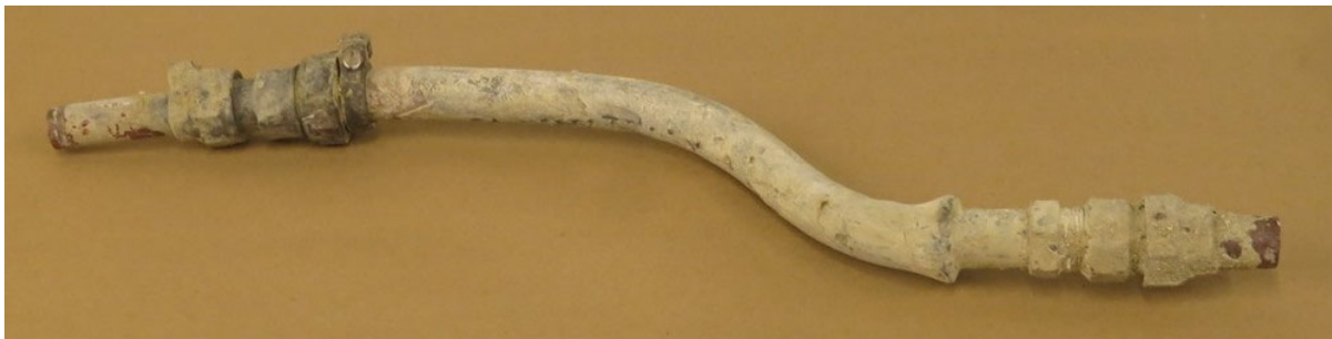
Figure A-5. Sample 16-0209-CP-1, Lead Pipe with Two Couplings Cu-Pb.
