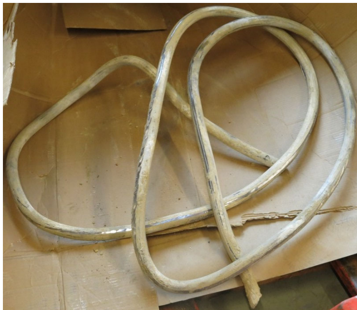
Figure A-3. Sample 16-0209-Pb-2, Lead Pipe.
