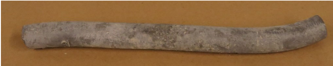
Figure A-2. Sample 16-0209-Pb-1, Lead Pipe.
