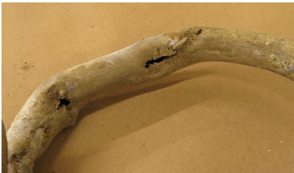
Figure A-17. Damages on the Lead Pipe from Sample 16-0209-CP-2.
