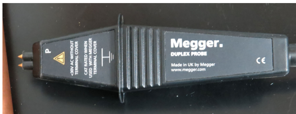
Figure 3-1. Megger Duplex Probe with Current and Measurement Potential Leads (Commercial Lead).
