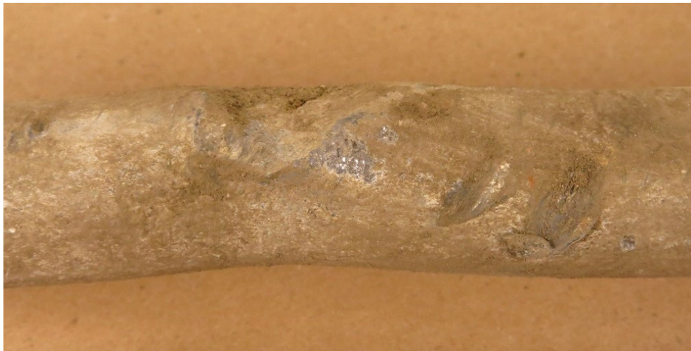
Figure A-16. Damages on the Surface of the Lead Pipe from Sample 16-0209-CP-2.
