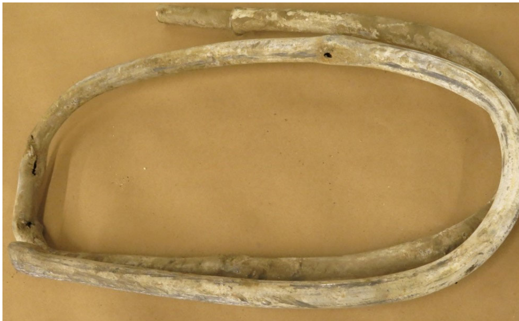
Figure A-6. Sample 16-0209-CP-2, Lead Pipe with One Coupling Cu-Pb.
